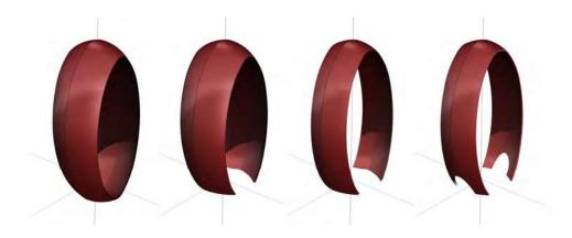
Figure 3 Shell including the horizontal elements was constructed using variable curvature steel arches braced together with linear members. The latter area was geometrically optimised to form flat quadrilaterals in order to be easily clad with rigid structural decking.
